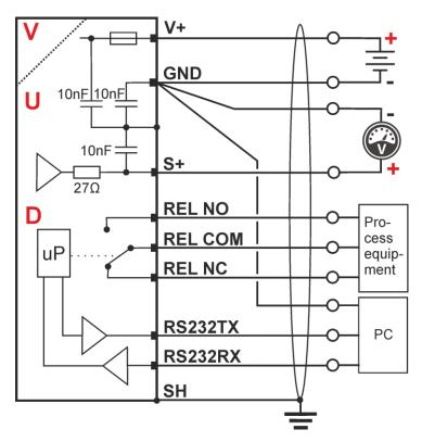
The high resolution 16-bit voltage signal can be interfaced to a PLC, A/D converter, voltmeter or other readout devices.
