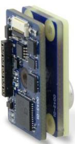
The MEMS SmartPirani™ heat-loss vacuum transducer for space flight use offers a measuring range down to 1E-6 mbar (7.5E-7 Torr) and is designed to withstand G-forces and vibrations experienced during rocket launch.
