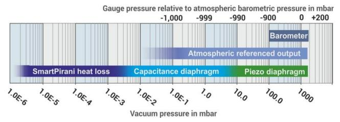
In environments where gas composition or type fluctuates, traditional gas-dependent Pirani gauges can result in measurement inaccuracies. The TriCAP™ ATM transducer integrates a high-precision capacitance diaphragm gauge (CDG) sensor, eliminating gas dependency and ensuring reliable measurements, even as gas properties change.
